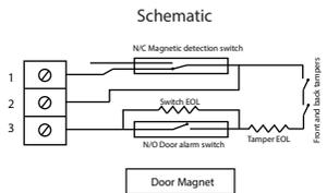
**Note: Wired as a single detector, at least one link from each row must be cut for this unit to function correctly**
